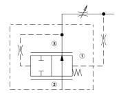
A screw-in, cartridge-style, load sense, flow-on-demand pressure-compensator.
