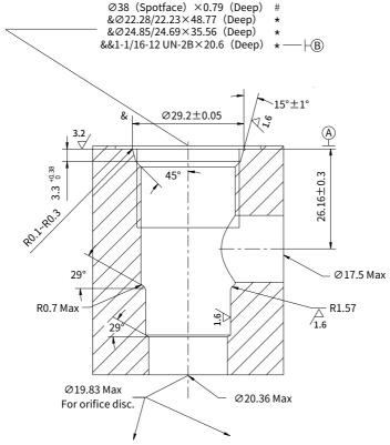
Note: Cavity variation 'A', \*\* pilot drill Ø19.05 Min., required to Min. depth of 54.4 from spotface.
