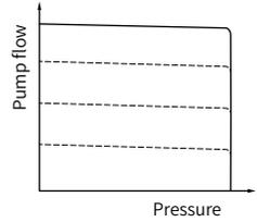
**Function and Features:** **Load sensing + Pressure Cut-off**
