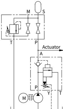
Hydraulic system with high and low pressure pumps
