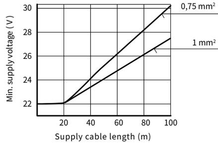
The minimum supply voltage of the power supply unit depends on the length of the supply cable (see diagram). In the case of lengths  $>50\text{ m}$ , a capacitor of  $2200\mu$  must be provided in the supply cable in the vicinity of valve.
